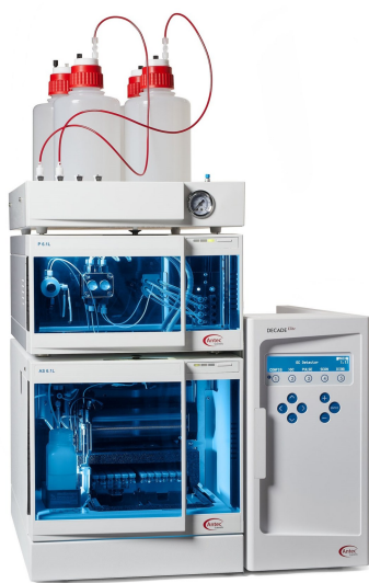
Figure 1. ALEXYS Carbohydrate Analyzer consisting of the ET 210 eluent tray (for N2 blanketing), a P 6.1L quaternary LPG pump, AS 6.1L autosampler, and the DECADE Elite electrochemical detector.
